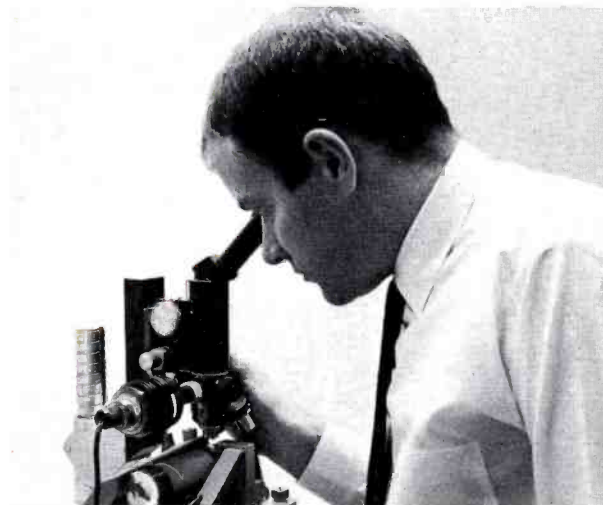
FIG. 6. Video head wear conditions can be evaluated by viewing the pole tips under a 150-power microscope with light attachment.
