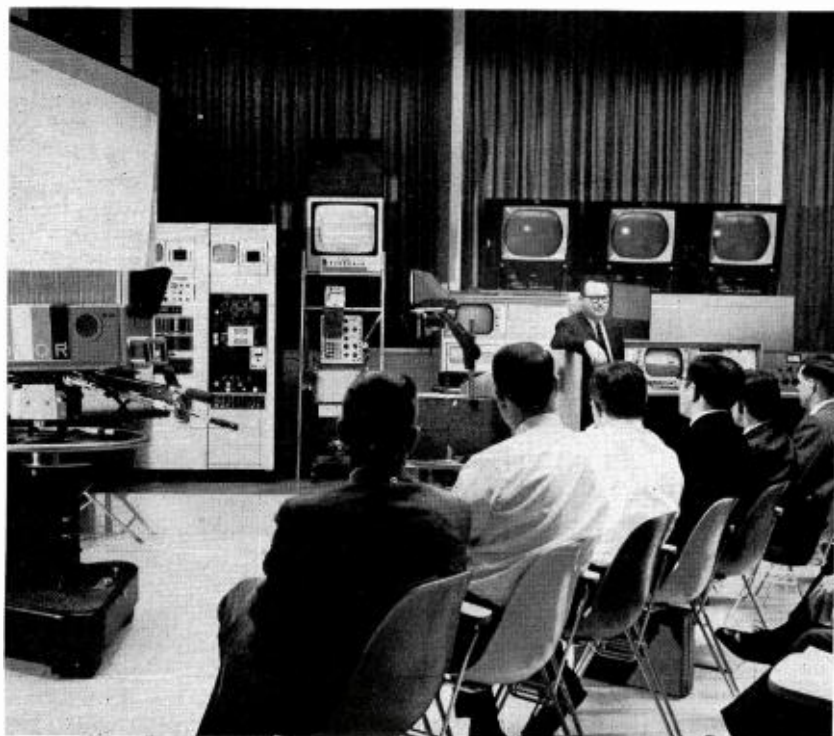
FIG. 2. Control room where studio and film camera operation is analyzed. Console includes full monitoring and switching facilities for video and audio. Color cameras are rolled into studio at left for live pickups.
